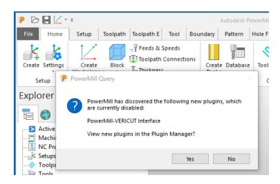
Click **File** tab > **Options** > **Manage Installed Plugins** to display the **Plugin Manager** dialog where you can manage the plugins that are installed on your PC.
